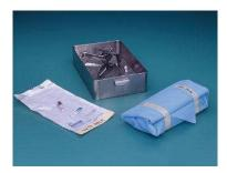
Place the Attest steam biological indicator and the Comply chemical integrator in the center of a suitable test pack or tray which is representative of the load and is the greatest challenge to the steam sterilization process.
