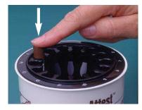
Push the activated indicator down to firmly seat in the metal heating block. Be sure the cap remains above the metal block.
