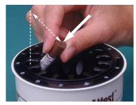
As shown, place the bottom of the biological indicator vial into the incubator's metal heating block so that the vial is at an angle of approximately 45°.
