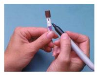
Identify the Attest biological indicator by noting the sterilizer number, load number and processing date on the label of the vial.
