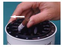
Push the vial straight back. This crushes the vial and activates the indicator.
